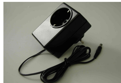
Pict. 6: Vacuum cleaner switch box
