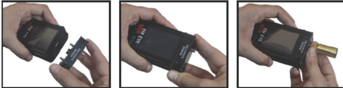
Figure 6. Attaching the sensor module to the EM Eye Meter
