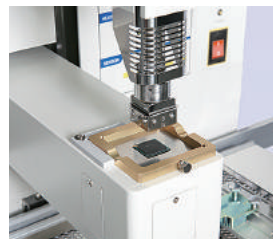
Place the CPS or AFD on the optic arm, press start and it will automatically pick the part from the tool, this automation prevents any smearing of the paste or the flux.
