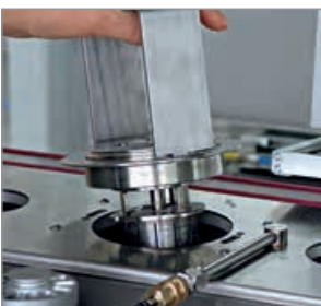
„QUICK RELEASE“ solder pump: Simply turn pump 45° and the pump is ready to remove
