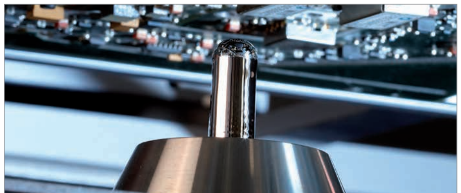
Soldering process with the wettable nozzle
