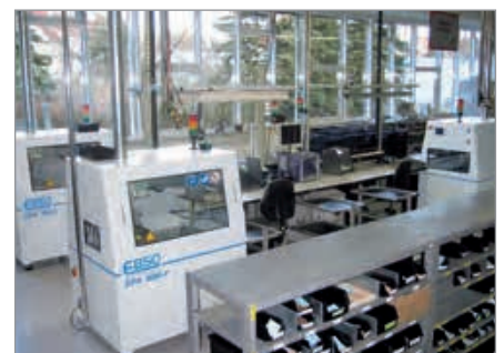
Production at Werma Signal Lights in Germany: 3 SPA machines, inbetween operator working place insures highest flexibility and throughput - always 3 different (or same) products are in production at the same time
