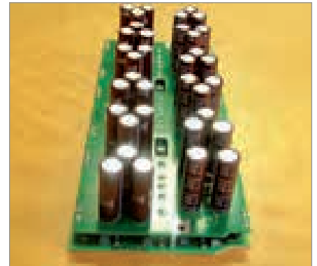
Selective soldering application with 45 mm interfering edge
