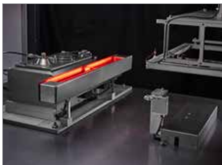
Processing room of the soldering system
